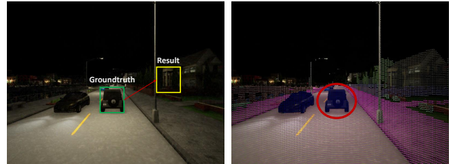
Figure 12: Effects of sensor fusion on attack results. Although the object tracker is hijacked (left), the original object still registers on the LiDAR (right, circled).
