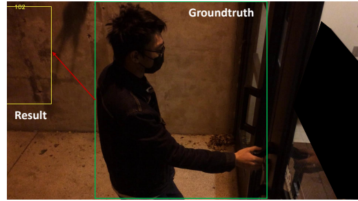
Figure 11: Noise cancellation resulting in unintentional tracker hijacking when no attack is conducted.
