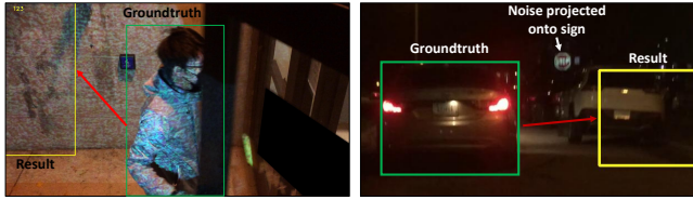
Figure 7: Offline move-out attack conducted on pedestrian (left), disguising his entry without setting of an alarm, and a vehicle (right), causing the victim vehicle to rear-end it.
